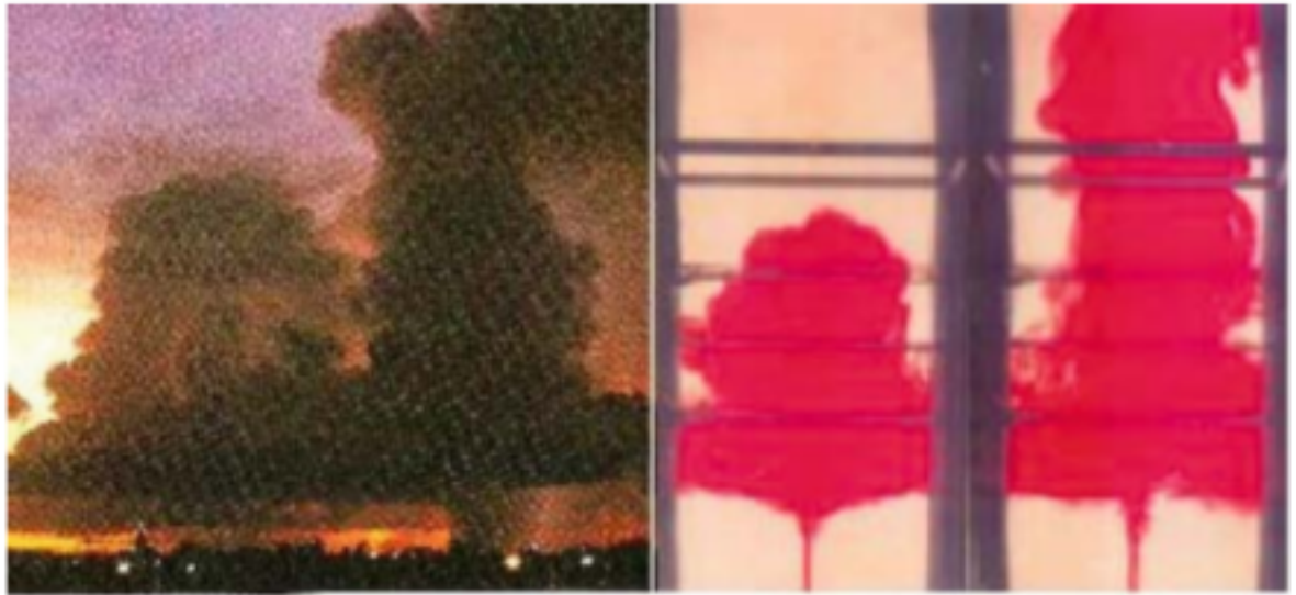
Figure 1.3: (a) Natural clouds. (b) Image from a dye flow visualization of a jet subjected to off-source volumetric heating, neutral with respect to ambient in the lower, denser layer below where the jet spreads out horizontally. (Narsimha and Bhat, 2008)
